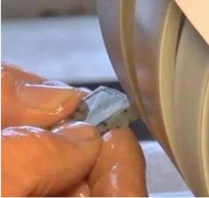
Hold the stone with the template mark parallel to the wheel, as shown. Slowly turn the stone keeping the wheel parallel to the template mark. Never use a fast motion. Do not slide the stone from left to right. This will cause flat spots.
