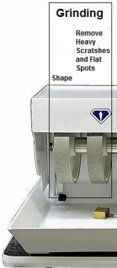
**The First and Second wheels are used to grind the stone to Size**
