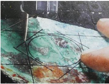
Start the cut by using medium pressure. Push the slab into the saw blade so the blade is just outside the “cut-line”. If the blade veers into the line, stop immediately and reposition the slab.
