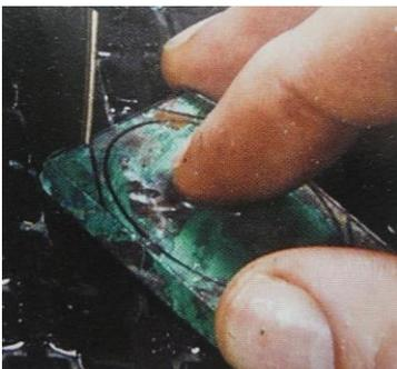
The more material that can be removed with the trim saw, the less time will be needed in the grinding process.
