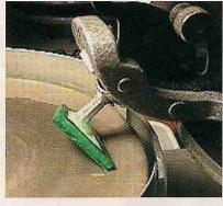
Remove the intarsia assembly from the faceting machine. Using the transfer fixture, bond another dop stick to the back of the intarsia assembly. After the epoxy has set, use a small torch to warm the metal dop stick attached to the front face so that it may be twisted off. Warning: warm the original dop stick only — just until the epoxy softens — do not overheat the intarsia.
