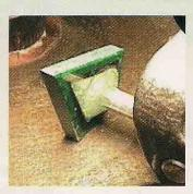
Reset the faceting machine head at 45° and grind a slight bevel on each back edge — bevels should be approximately ½6" wide. Using the polishing procedure, bring each bevel to a final polish.
