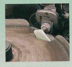
(96 or 0 less 30 divisions = 66 division mark). Using a 180-grit diamond lap, grind the long edge flat, then reposition the index wheel to the 30 division setting (0 plus 30 divisions = 30 division mark) and, without changing the depth setting, grind the other long edge flat. Note: Always work to the same depth-setting stop on each side of the centerline as this will insure the same angle and length of each side.
