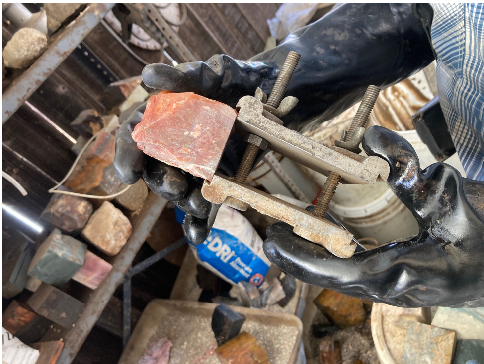
(another type of jig used to hold thick slabs or "end pieces" that need to be cut in order to utilize more of the rock.)
