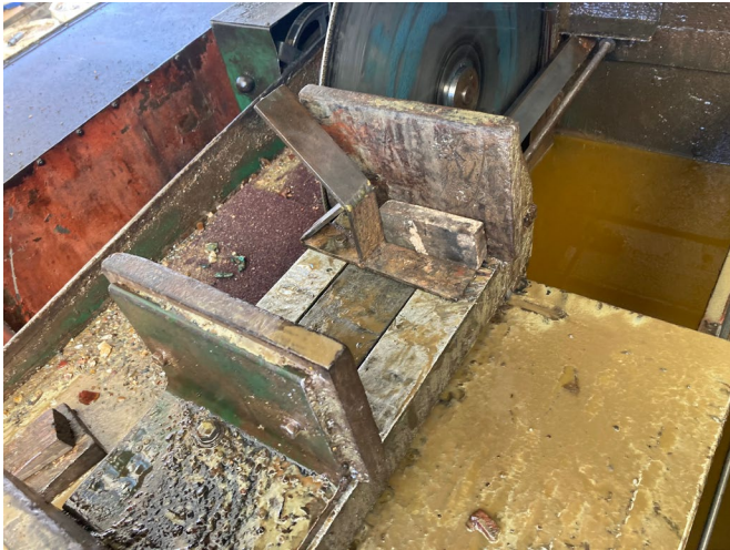
(one of the "jigs" Wes uses to make the 45 degree cuts.)
