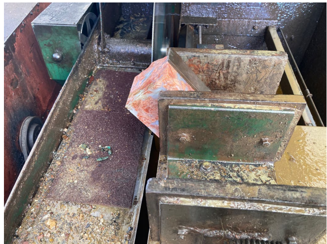
(the jig holding a cube of "Cotton Candy" rock preparing to cut off the edges at 45 degrees.)
