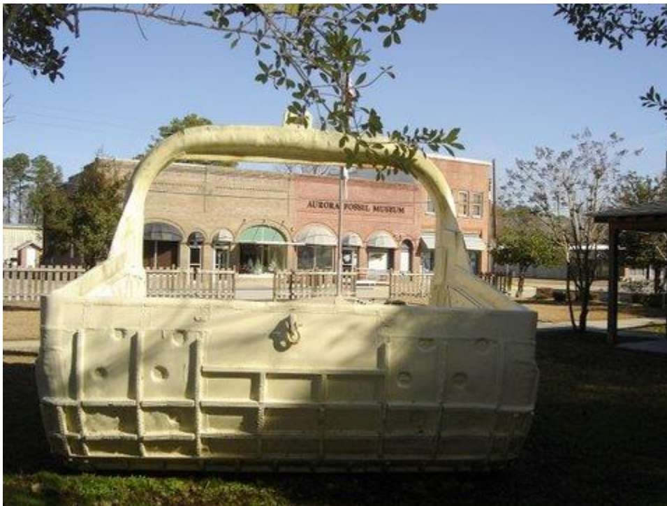
This is one of the old "dredge" buckets from the PCS Phosphate Mine. It is HUGE --- a sign on it says the bucket could dig (in one day) the equivalent of 25,000 pickup truck loads of material.
