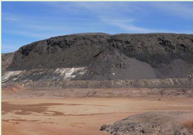
Pictured is a slag pile at Broken Hill in New South Wales. Slag is a man-made waste product created during smelting. Credit: Anita Parbhakar-Fox
