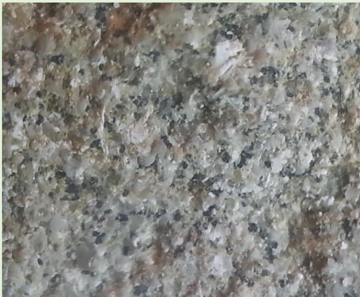
Calcareous sandstone containing glauconite (dark colored) granules, Prince George's County, Maryland
